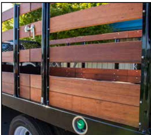
Flatbar Rail and Flatbar Supports 2" x 3/8"
